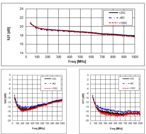
V<sub>c</sub> = 3.3V, I<sub>c</sub> = 50mA, T=25°C
