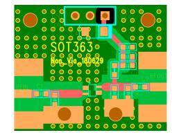
\*Dielectric constant \_ 4.2 \*RF pattern width 52mil \*31mil thick FR4 \*Without vias under device degrade device performance.
