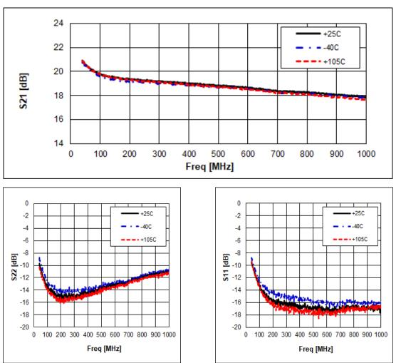
V<sub>c</sub> = 3.3V, I<sub>c</sub> = 50mA, T=25°C
