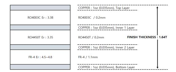
Figure 31. Evaluation Board PCB Layer Information
